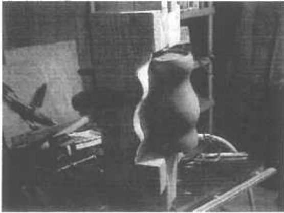
The wet leather stretched around the wooden former and clamped in place using profile cut boards.
